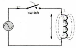
**Inductors**: are coils used to oppose the changes in electric current (AC) in a circuit. They are used to reduce current in a circuit without energy loss.
