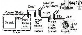
In our country, electricity is generated at <u>11kV</u> and is supplied to household users at <u>230V</u>. A step up transformer is used at <u>power station</u> to increase AC voltage from 11kV to 220kV. Step down transformers are used in all other stages.
